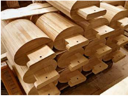
Details of precision CNC-milled components
